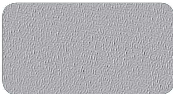
thin worms standard pattern on unprinted alu foil (enlarged)
