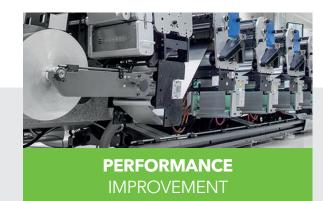
Formika is one of Poland's first companies to have had, since mid-2016, a press equipped with a nitrogen atmosphere printing technology that delivers faster printing speed (for improved efficiency) and reduces migration with the same installed capacity of UV lamps.
