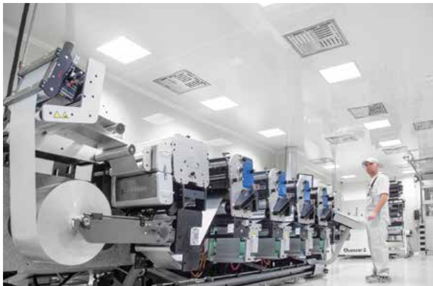
The class D cleanroom (ISO 8) is where aluminium packaging for medicines is produced. The entire production process, starting from printing, slitting and winding, all the way up to packing, takes place in sterile conditions. A new Gallus printing machine stands in the cleanroom.
